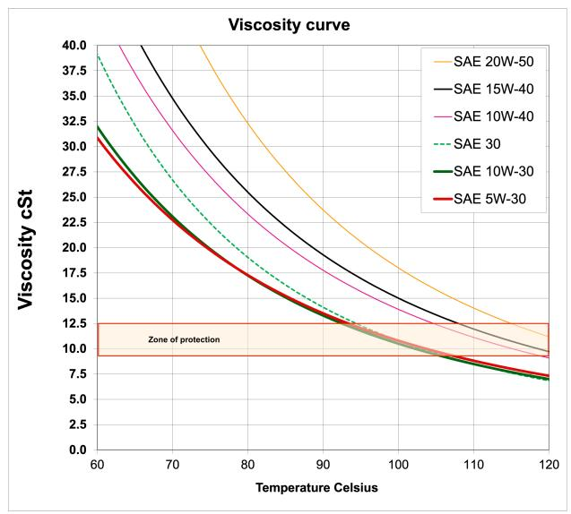
You can see from this chart that until the engine reaches operating temperature there is very poor lubrication and frequently the oil is going through the bypass valve directly to the bearings without passing the filter (in other cars it goes through the dirty filter and out the bypass valve). During this period, you should refrain from putting the engine under high load or high rpm.
