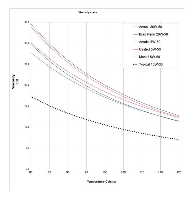
Before considering a 5W-50 oil, you should look for its HTHS value. There is no point in a higher viscosity that shears down below the 5W-40 oils on the market, and we should remember that our Corvairs should be lubricated with 10W-30 under most circumstances. You do not want an HTHS higher than the engine design, as it will cause pitting or other wear in the bearings.
