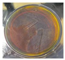
ready for anything. The oil in this picture is from a new car, with 2000 miles on it. There are thousands of shiny particles floating in it, even though it had an EOM oil filter.
