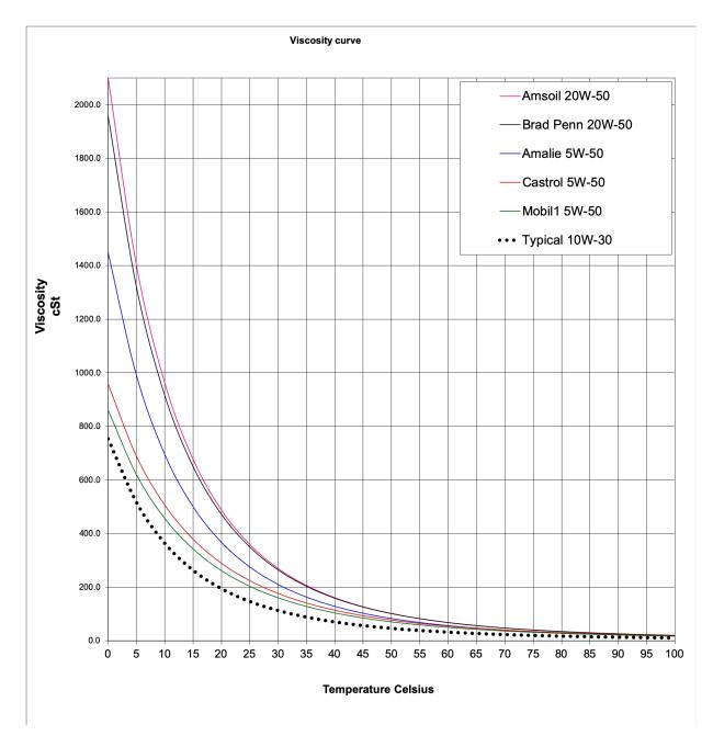
Note that in these graphs, I have added a dotted black line for the viscosity curve recommended by Chevrolet for the Corvair. Anything thicker is not fully flowing and protecting.
