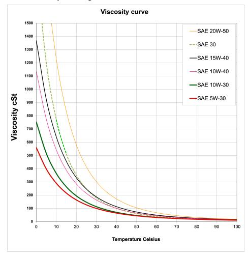
Here is the same chart, looking in detail at the viscosities at the high end of the operating temperature range. You will see that around 80°C (176°F), the 5W-30 is more viscous than the 10W-30, giving more protection at both ends of the scale. There will be slight variations between different brands.
