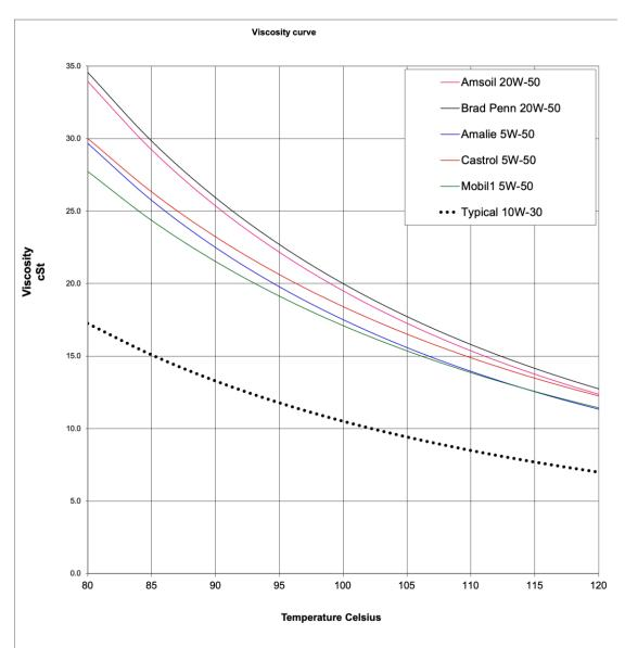
The second graph shows the viscosities of the same oils at operating temperatures.
