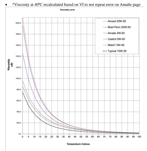
Note that in these graphs, I have added a dotted black line for the viscosity curve recommended by Chevrolet for the Corvair. Anything thicker is not fully flowing and protecting.
