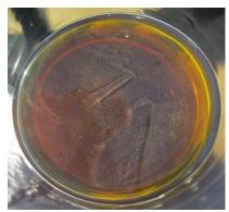
ready for anything. The oil in this picture is from a new car, with 2000 miles on it. There are thousands of shiny particles floating in it, even though it had an EOM oil filter.
