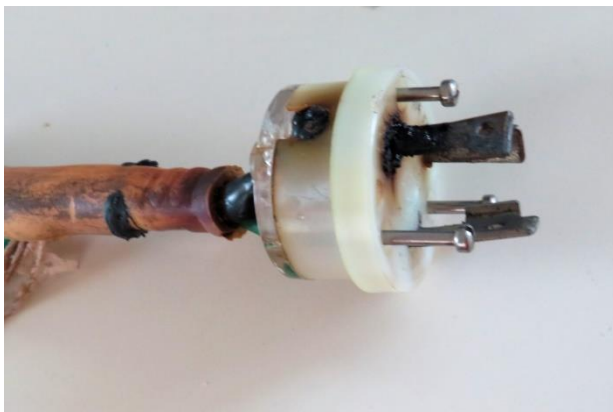
The "guts" of a burned electric plug
